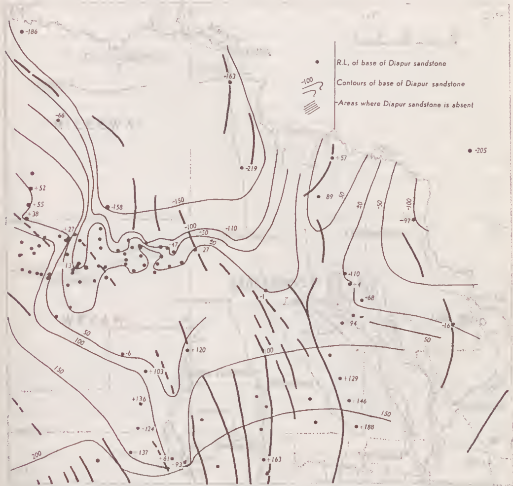
FIG. 6—Structure contours of the base and the position of the main ridges of the Diapur Sandstone in the Mallee Region. Note, this formation is absent in the SE. corner.
